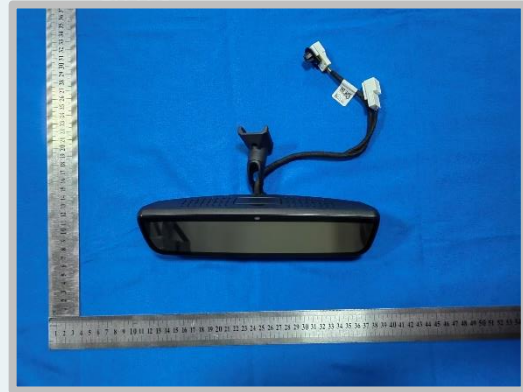
After test (The reflecting surface is not break)
