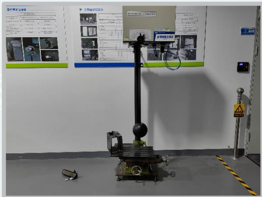
After test (It fell off on impact, mirror intact)
